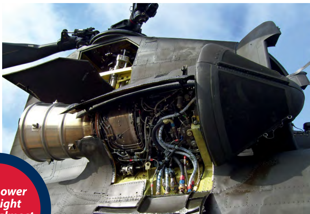
Above: A Lycoming T55-GA-712 turboshaft engine on a CH-47 Chinook. Image by 'MrZ-Man', CC BY-SA 3.0.
