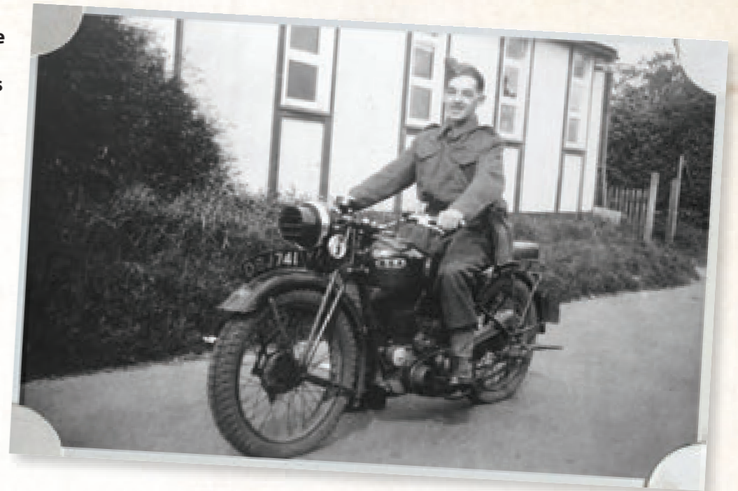
Doug in 1941 during his time with the Home Guard. The cover on the motorcycle’s headlamp made detection by enemy aircraft more difficult. © Doug Vince
