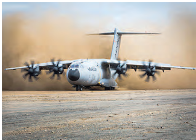
UK - A400M Sand Surface Landing Trials, Woodbridge. Photo: © MoD/Crown
