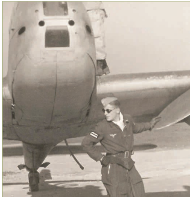
A rare head on shot of the 210 showing the under nose bomb doors. Photo: © Author
