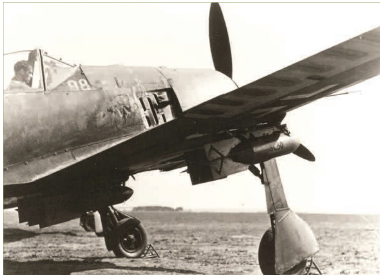
A good view of the bomb rack positions with 50 kg bombs under the wing. Photo © Author
