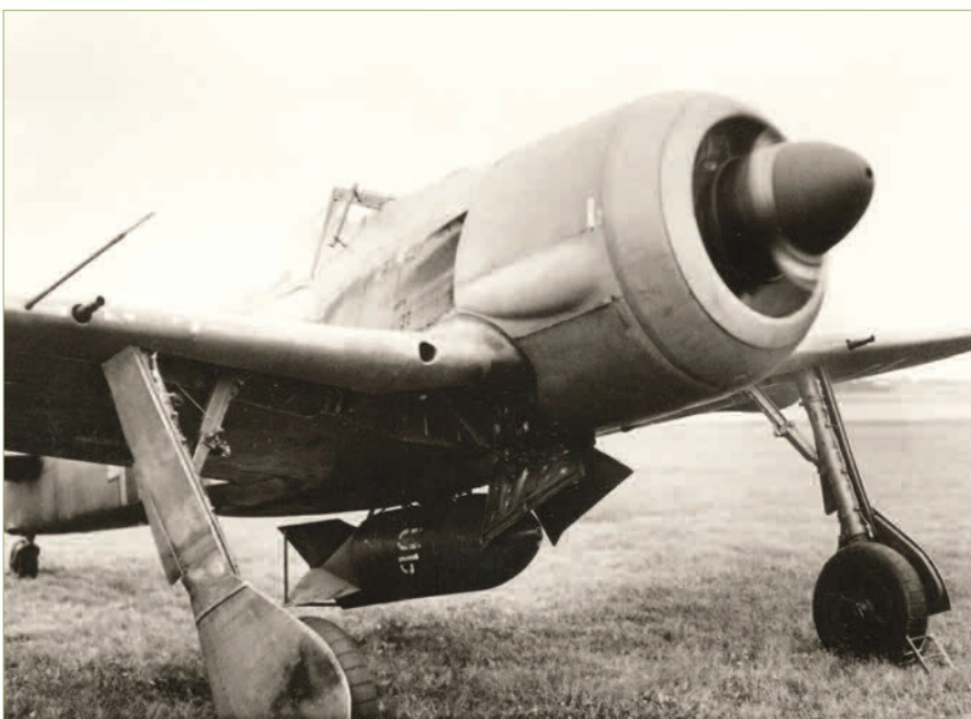
Another good view showing the of central bomb rack position of this fighter bomber. Photo © Author
