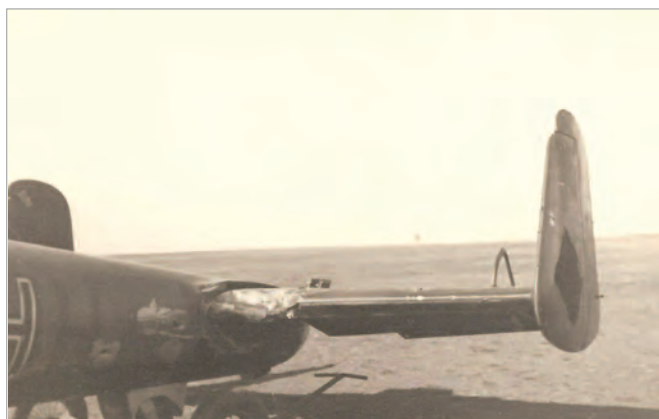
Above two pictures of Oberfeldwebel Hagen's Do 17 at Brest after being damaged by 611 Sqn; the damage to the tailplane was caused by the crew member that baled out and hit the tailplane. Photo: © Author.
