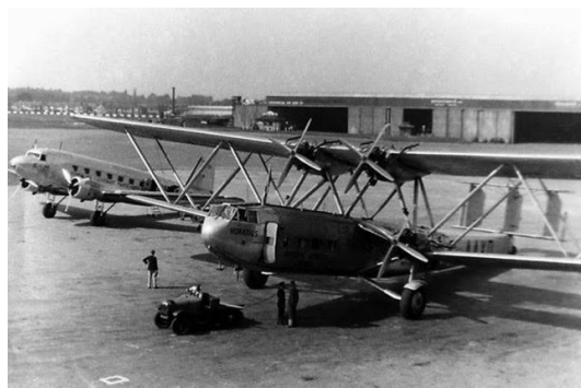
Picture 14. Imperial Airways at Cairo. 1932. Note the refuelling equipment, including the ladders resting on the upper engines. Note, also, the modest terminal
