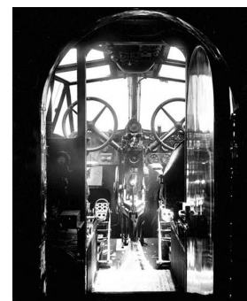
Picture 9. The cockpit of a Handley Page HP-42 airliner. London, 1931. No powered controls here.
