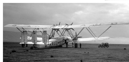
Picture 11. HP-42s at Croydon. Part of the Co-Pilot's duties was to stow the flag before take-off. The Bristol Jupiter engines are warming up.
